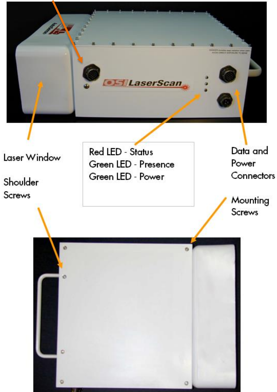
Figure 8: AutoSense™ Enclosure Detail
