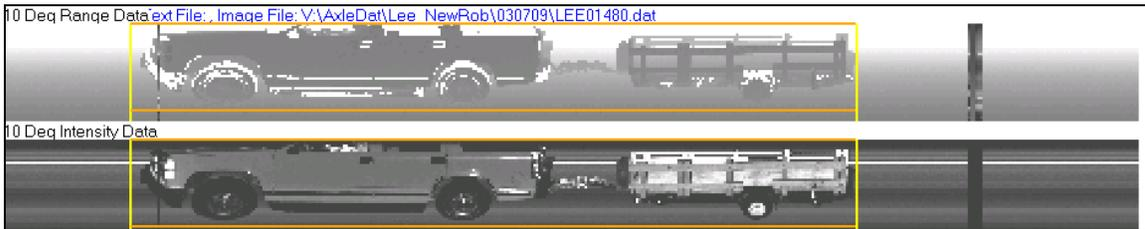
**FIGURE 0.3 3-D Range Image of SUV Towing a Trailer**
