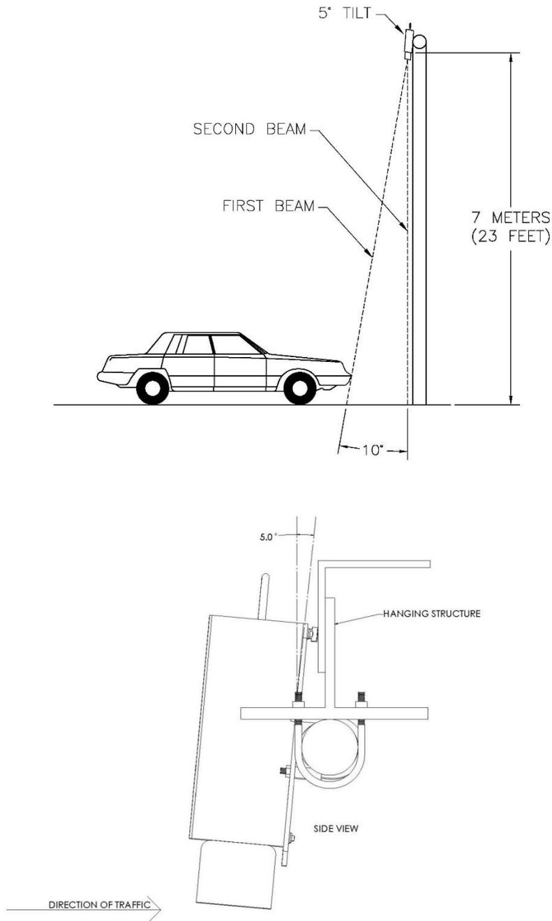
**Figure E-1. Overhead Mounting and Look Down Angle**
