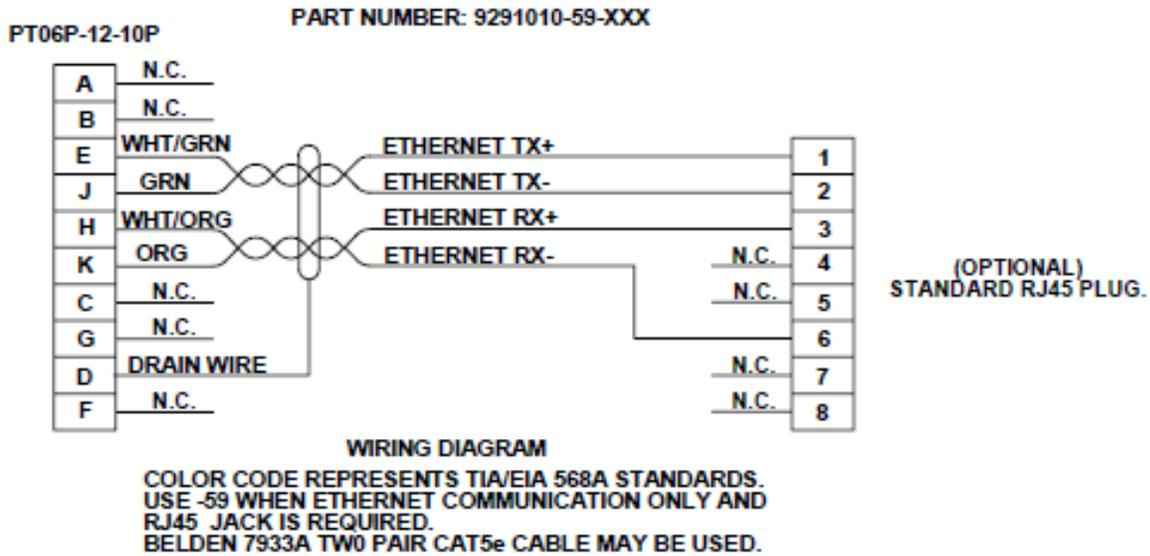
**Figure 17: Front Port Ethernet Data Communications Cable Schematic**
