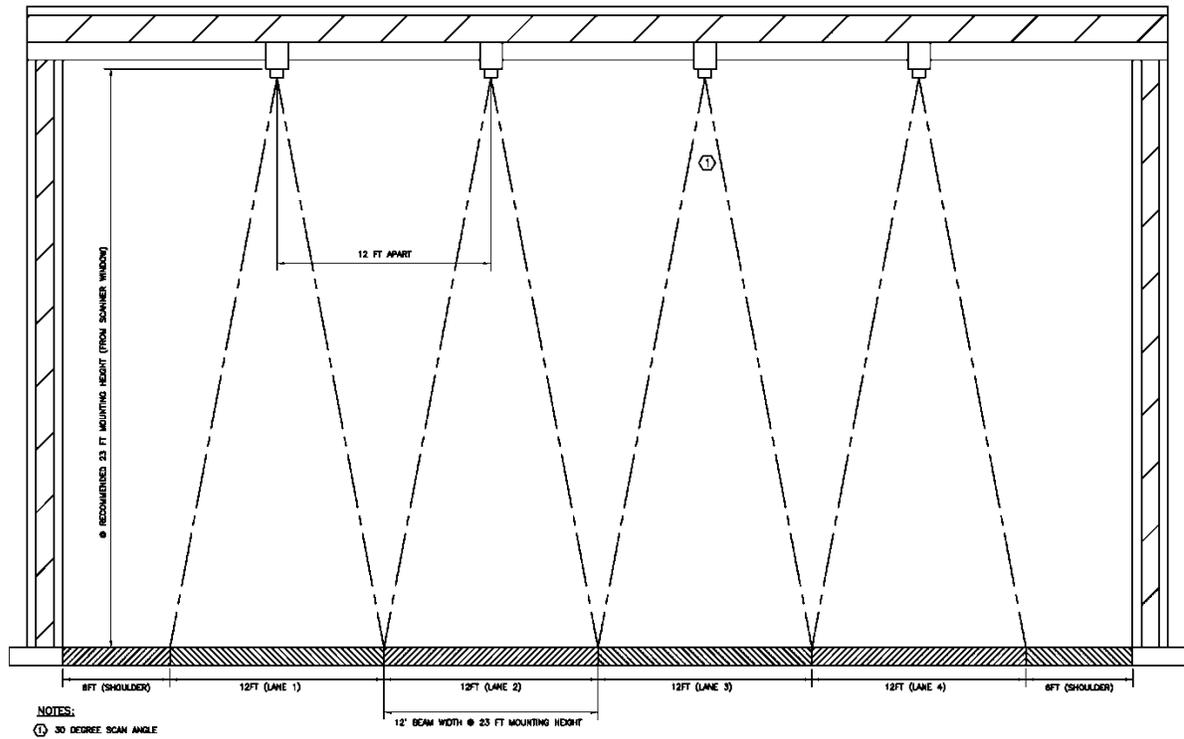
Figure E-5 Elevation of Typical AutoSense Open Road Installation at Center of Lane
