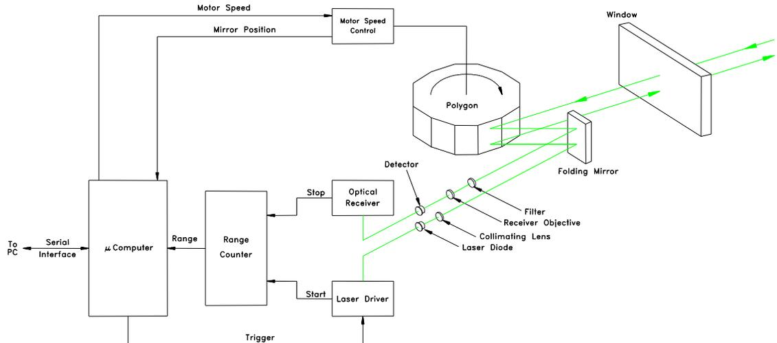
**Figure 2: AutoSense™ System Schematic Diagram**
