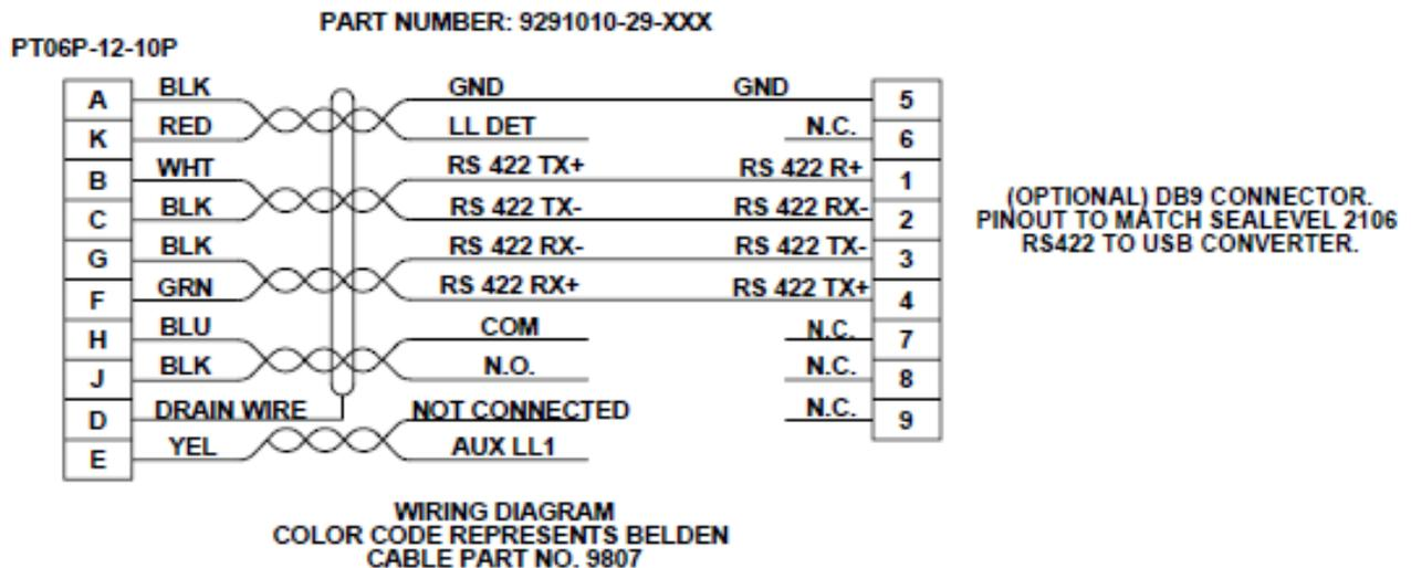
Figure 15: RS422 Message Data Communications Cable Schematic
