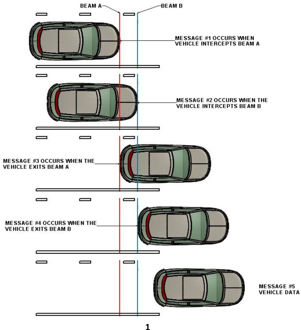
Figure 13: AutoSense™ Output Messages versus Vehicle Location.
