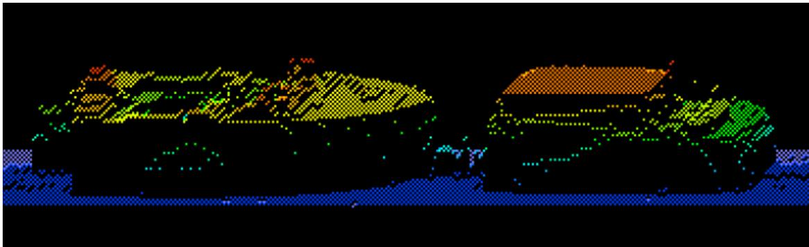
Figure 5: 3-D Range Image of Van Towing Boat
