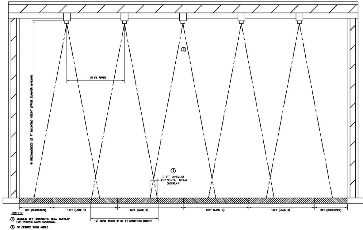
Figure E- 4 Elevation of Typical AutoSense Open Road Installation with Shoulder Coverage
