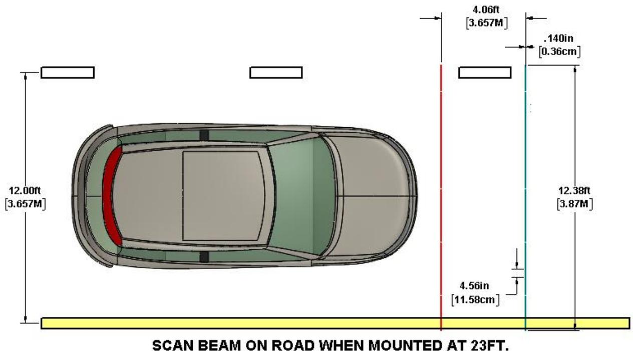
Figure 6: Laser Beam Footprint on Road Surface
