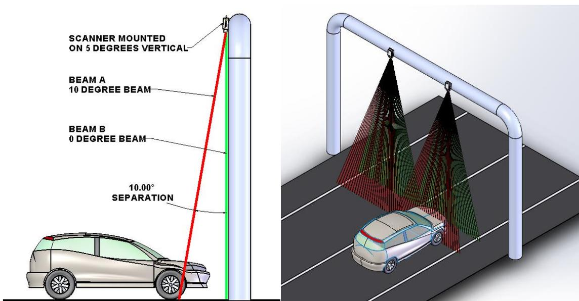
**Figure 3: AutoSense™ Beam Scan Geometry**
