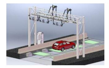
Using information gathered from loop data, Neology Idris AVC provides a record of each vehicle that transits through the loop array. These records are known as Per Vehicle Records (PVRs); PVRs provide important information on a vehicle's speed, length, class and number of axles. Vehicle classes are defined during system configuration and can be easily altered to suit a tolling agency's requirements.
